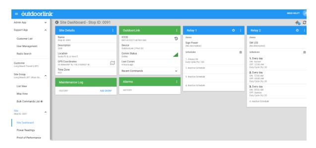
10. If the schedule is set for *Always On,* or the Relay is scheduled to be on at the time, the device should power up once the controller receives power and connects to its cellular carrier. If the schedule is not set to be on at the time, then push the Power Button located on the blue header of each Relay:
